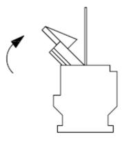
Once the cable has been inserted carefully close the connector.
